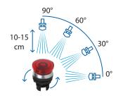
**IP 69K:** against water jets with high temperature and pressure
