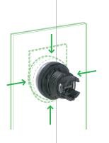
**Auto-grip ring** head held firmly in the drilling hole during assembly
